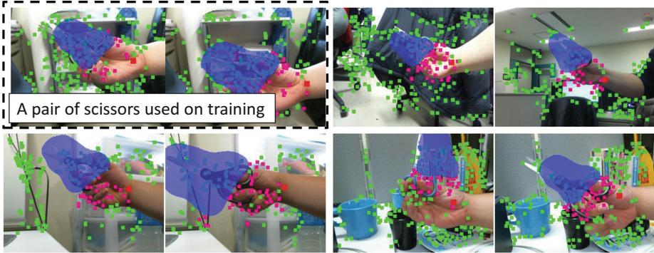
**Fig. 13.** Results for a hand grasping a scissors not used on training
