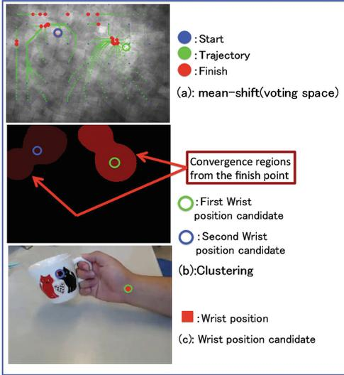
**Fig. 2.** Flow of wrist candidate detection (Color figure online)
