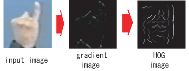
Figure 2. Example of HOG Feature. Left:Input Image, Center:Gradient Image, Right:HOG Image
