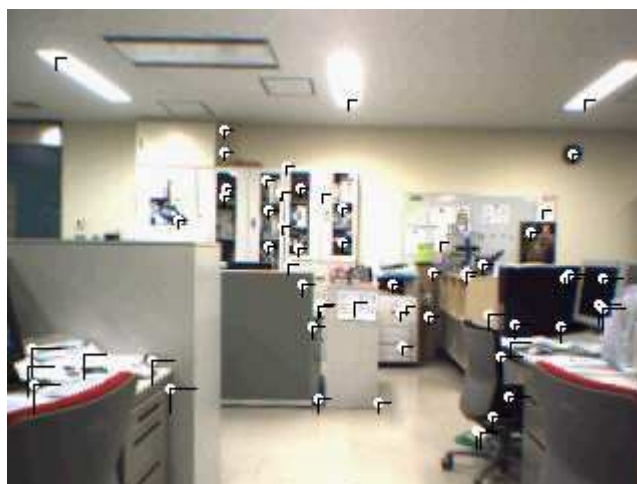
Figure 1 Trinocular correspondences: The white filled circles are the stable keypoints, the black lines from the stable keypoints are horizontal and vertical disparities.
